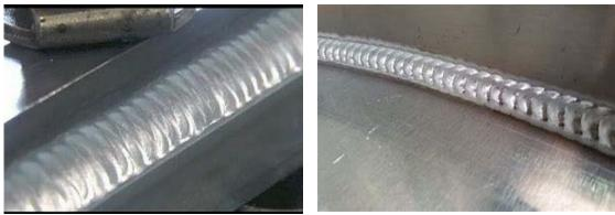
Pulse MIG welding can be used to both thick and thin aluminium, on thicker sections, it helps minimize downtime for repositioning parts since it generates a cooler weld pool than traditional spray transfer process, making it usable in all welding positions.
